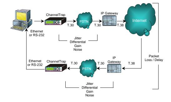
The analog connections through the PSTN are subject to phase and amplitude jitter, as well as differential gain and circuit noise. FaxLab employs a measure of modulation symbol quality called the Eye Quality Monitor (EQM) that provides a qualitative value for these effects on transmission quality. Internet transmissions can incur excessive packet delay and outright loss. FaxLab performs an end-to-end comparison of signal delay to milliseconds and signal content to the bit level.
